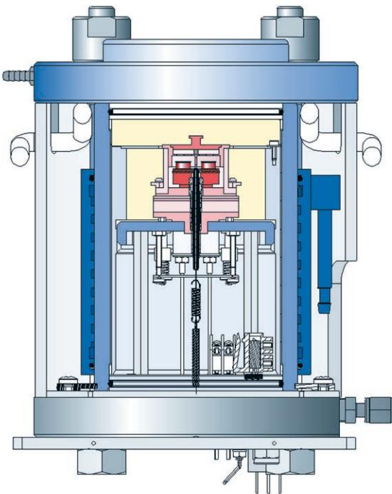
In the HP DSC 2+, the low-inertia, fast heating/cooling DSC furnace is incorporated in a water-cooled pressure vessel. The furnace is specially insulated so that no temperature gradients occur. This guarantees a stable and reproducible baseline, even at higher pressures.
