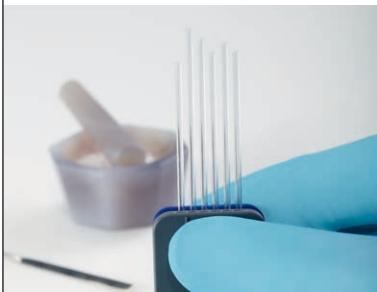
Sample preparation can be time-consuming. Our innovative sample preparation tool holds up to six samples and simplifies the correct filling process. Its unique design allows you to insert the capillaries directly into the instrument.
