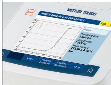
Automatic detection of transmitted light combined with video observation ensures that the melting, slip melting, boiling, and cloud point measurements are reliable. Statistical evaluation with standard deviation and mean value allow you to have full confidence in your data.
