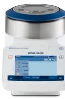
The MP70 is the perfect choice for melting point and melting range determinations.
