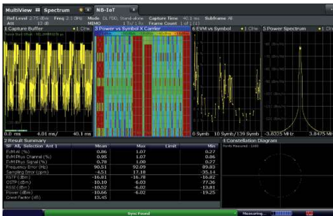
The R&S®FSW-K106 NB-IoT measurement application
