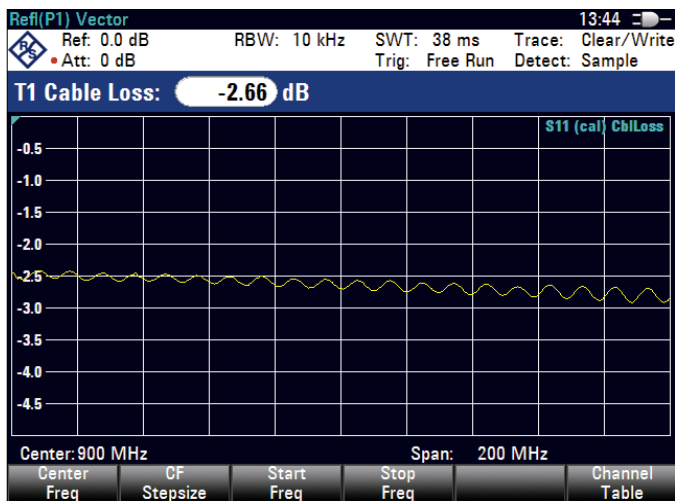
One-port cable loss measurement
