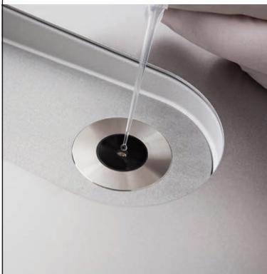
Micro-volume UV/VIS measurement is the method of choice when measuring either small sample amounts or high absorption samples. Only 1  $\mu$ L of sample is required for reliable measurements. The pure sample is pipetted on the measuring surface and the arm is locked automatically to a precisely defined pathlength. Measurement errors are avoided, as the sample does not need to be diluted.
