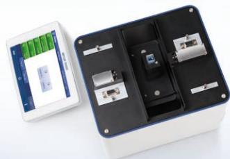
Exceptional ruggedness and reliability, thanks to the lack of moving parts in the optical section, long-lasting Xenon flash lamp and state-of-the art optical fibers. Their flexible connectivity to printers, PC, storage devices and barcode scanners, make UV/VIS Excellence instruments a sound, sustainable investment for the future.
