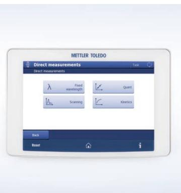
Spectrum scans, fixed wavelength absorption measurements, quantification with calibration curves or kinetic analyses are ready to use as direct measurements: Simply enter parameters, define the preferred workflow, store as a shortcut, and start the measurement with One Click.
