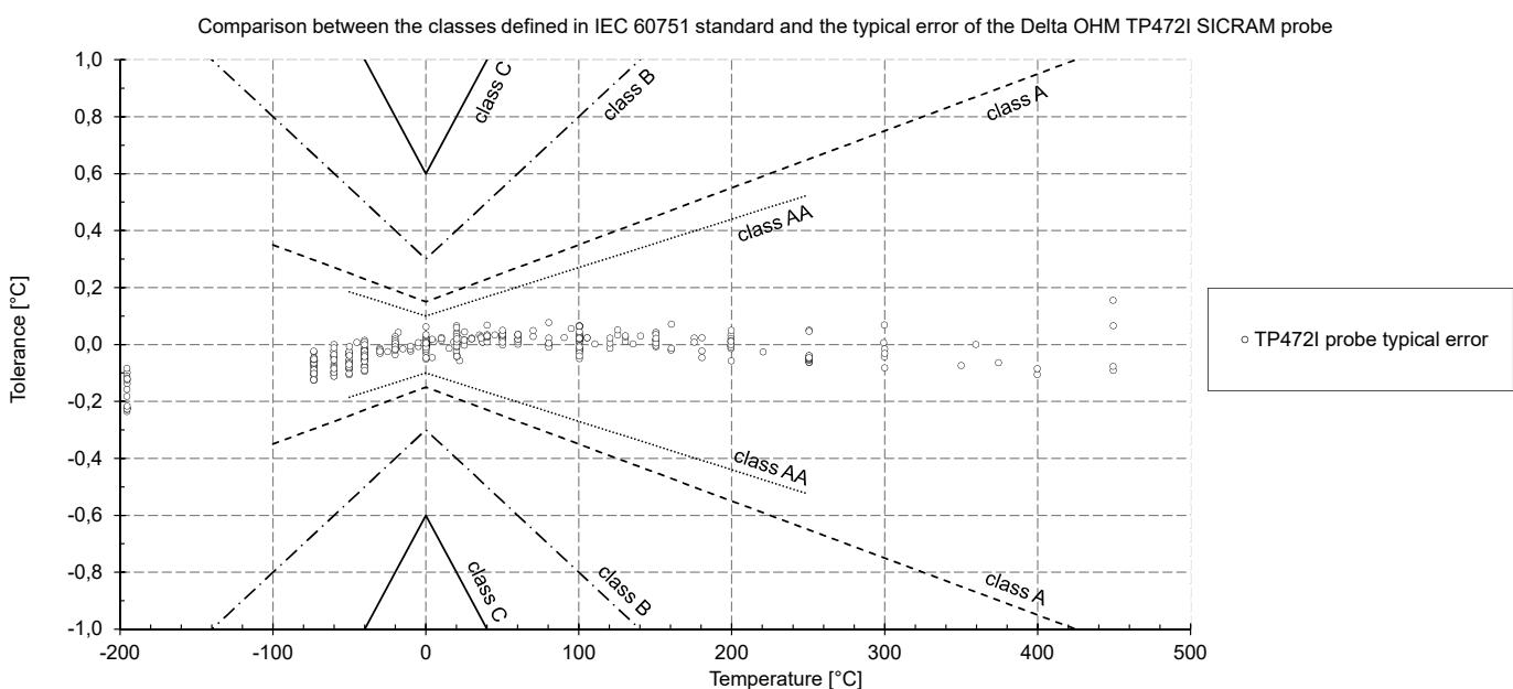
Tolerance as a function of temperature. The temperature range refers to the platinum wire wound probes.
